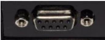
The controller is fitted with a D Sub 9 Pin Female jack.
