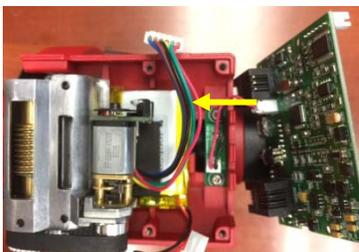
6. Rotate the RA axis to find two set screws next to the LED board, which are used to secure the polar scope in place. Use a hex key to release the set screws. Pull the polar scope out of the RA axle.
