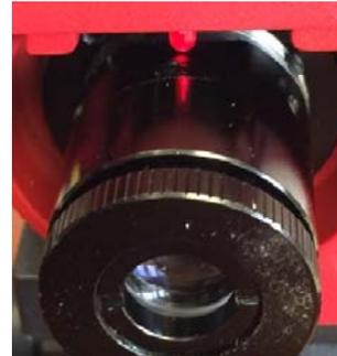
9. Insert the iPolar into the RA axis. Lock the set screw gently to secure the iPolar.
