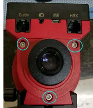
8. Remove the polar scope out of the RA axis.
