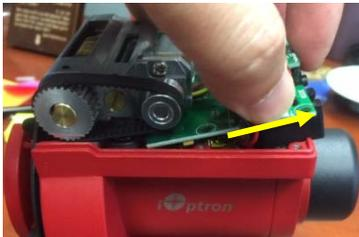
5. Disconnect the polar scope LED cable.
