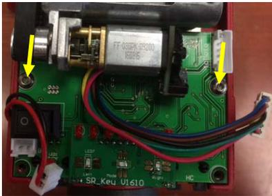
4. Gently pull the circuit board with sockets end up and slide the circuit board out.
