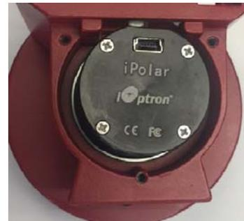
10. Replace the Polar Scope base plate with a new one with larger opening.
