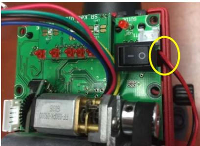
13. When securing the board with two screws, make sure that the battery and wires underneath are properly seated. Fully tighten the screws.
