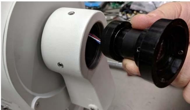
8. Slightly tighten two set screws on iPolar CEM60 adapter to secure the iPolar inside the RA axle.
