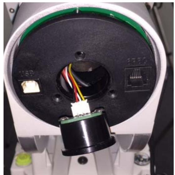
11. Insert the iPolar USB adapter into the RA axle through the CMS input panel. Lock it by tightening the set screws.
