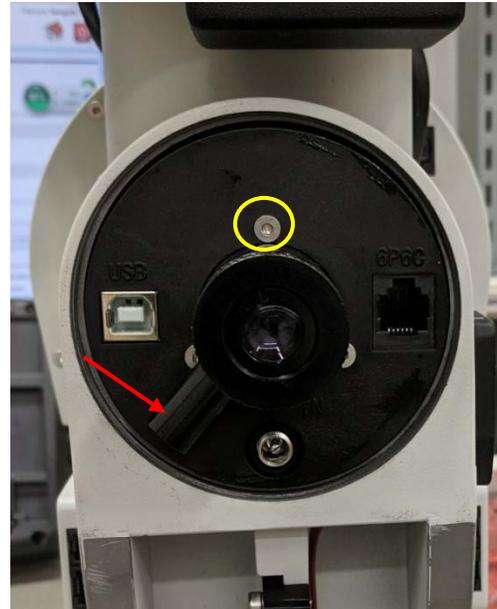
4. Pull the CMS input panel so a 1.5mm allen wrench can be inserted. Find two set screws that separated ~90 degree from each other on RA axle that hold the optical polar scope. Slightly release the set screws so the polar scope can be pulled out.
