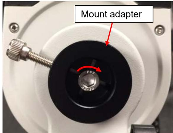
3. Install camera adapter. Finger tighten the locking screw on the mount adapter to secure it.
