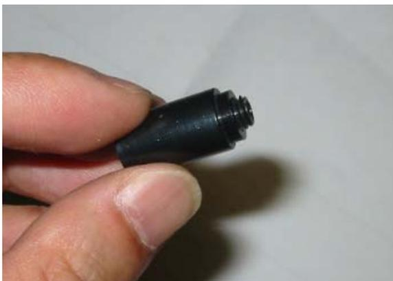
7. Loosen the set screw that holds the polar scope and remove it from RA axle.
