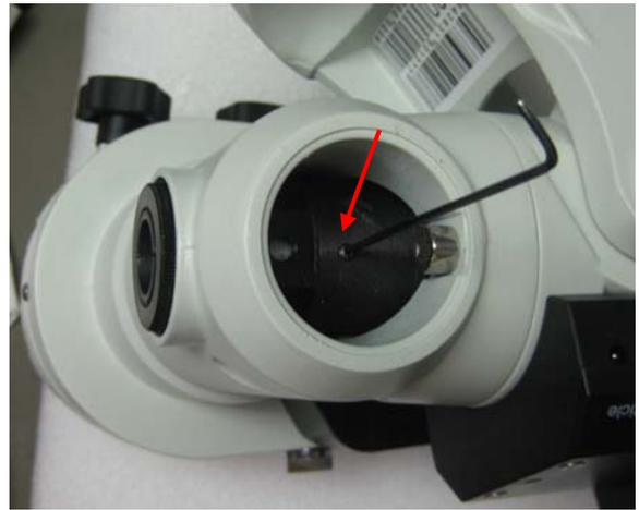
8. Insert the iPolar into the RA axis. Lock the set screw gently to secure the iPolar.
