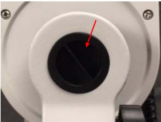
2. Insert iPolar mount adapter into the RA axle opening. Tighten the hex screw to extend the stainless steel adapter to secure it inside the RA axle.
