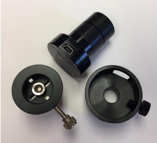
iPolar electronic polar scope **#3339-025** is designed for ZEQ25/CEM25 mount. It can be installed in front of the mount to keep the optical polar scope in place (front mounting), or at the back to replace the optical polar scope (internal/rear mounting.)
