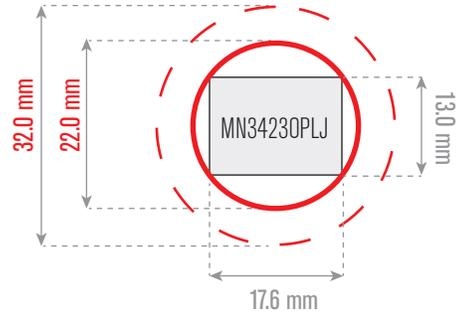
**Matrix Spot Diagram (18 µm box size)**
