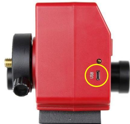
Figure 5. Micro USB powering/charging port
