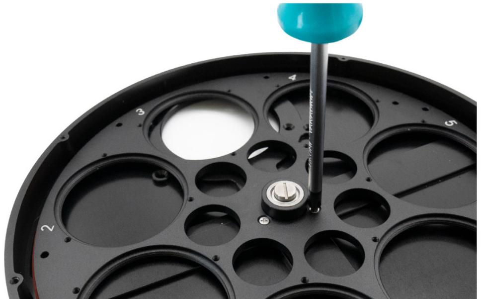
4) Align the four screw holes of EFW with these in the four corners of the camera chip as shown below:
