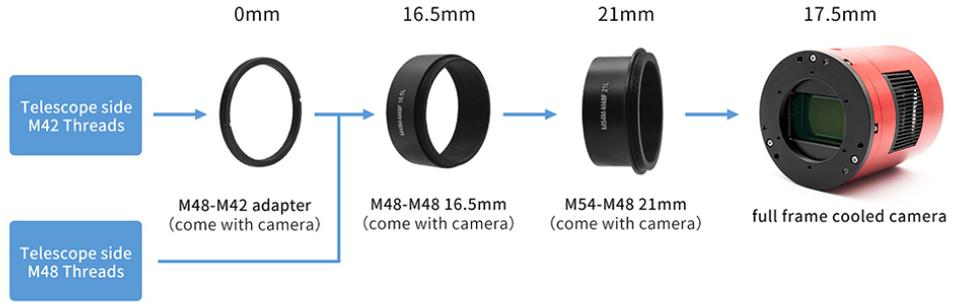
This solution needs the M48-M48 16.5mm extender and the M54-M48 21mm extender. You can find them in the package of the ASI6200 camera.
