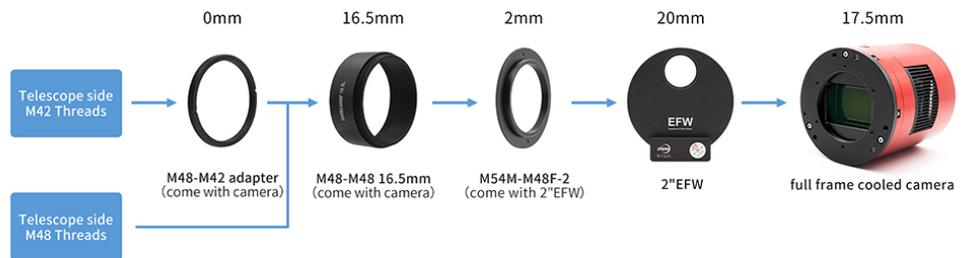
This solution needs M48-M48 16.5mm extender and the M54-M48-2 adapter (come with the 2" EFW). You can also buy the M54-M48-2 adapter separately.
