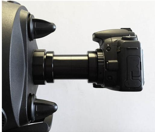
For use at  $f/7$ , remove the spacer and thread the filter holder back on to the shorter configuration as shown below. The T-ring should be threaded directly onto the filter holder.
