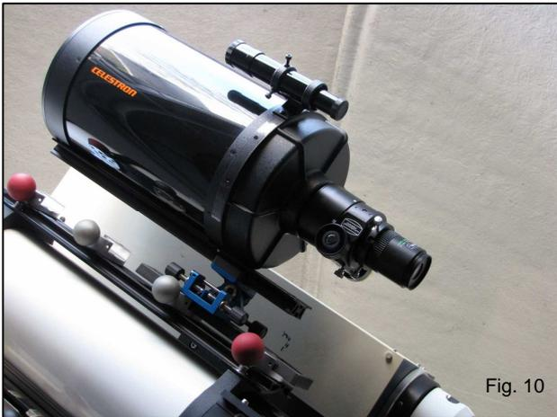
Fig. 10: C8 and Baader Steeltrack focuser with Stronghold
