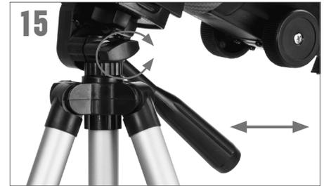
To move the scope right and left, hold a tripod leg with one hand while the other hand uses the panning handle to move the scope. The azimuth locking screw can be loosened or tightened to adjust the tension to your preference.
