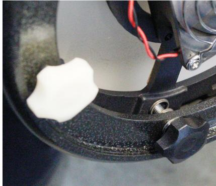
There are three white and three black knobs. Behind the black knobs, small springs can be seen. These are the springs that we will be replacing.
