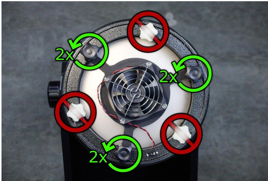
**DO NOT FULLY REMOVE THE SCREWS AT THIS POINT. NEVER REMOVE ALL THREE AT ONE TIME. If they are all removed at the same time, the primary mirror will fall out into the telescope and could be damaged.**
