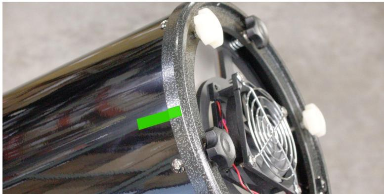
Mark the rear plate and OTA with a piece of masking tape, so that they can easily be reassembled in the same orientation.
