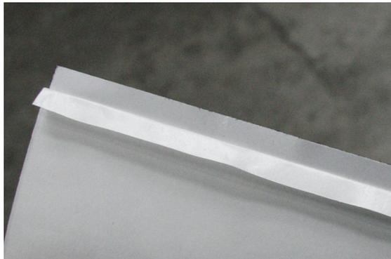
Roll the flocking paper and position it inside the optical tube (OTA) where you want it to sit, and then gently press down along the edge where the adhesive back is exposed. Now that the edge is adhered to the OTA. Slowly peel back the paper backing while pushing the flocking paper against the inside of your telescope, sticking it in place.
