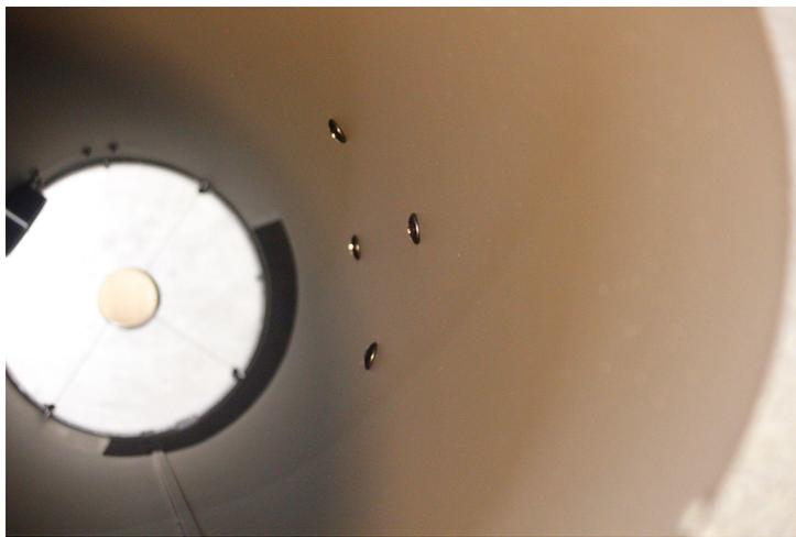
Just like the upper flocking, use one of the wet cleaning wipes provided in the kit to clean the inside of the OTA. Clean just past the screws that you can see about 15" up the tube. *When installing the flocking, it might cover these screws. This is ok and on some models it is unavoidable.*
