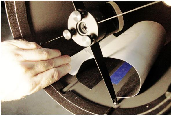
If any wrinkles or lines form, do not be discouraged. These are only cosmetic and the flocking will still perform incredibly well. A utility knife can be used to cut the paper releasing air trapped behind the flocking or to help smooth wrinkles or folds.
