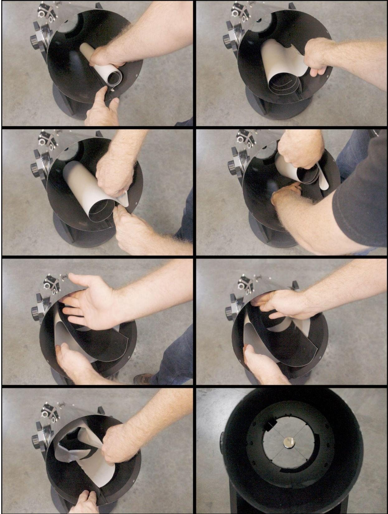
Once the flocking is in place, the primary mirror assembly will need to be reinstalled. Take note of where the masking tape alignment marks are. Gently install the assembly back into the OTA maintaining contact with it at all times until several of the screws are installed. If someone is available to lend a hand, it could be beneficial here. Do not fully tighten the screws until all have been started.
