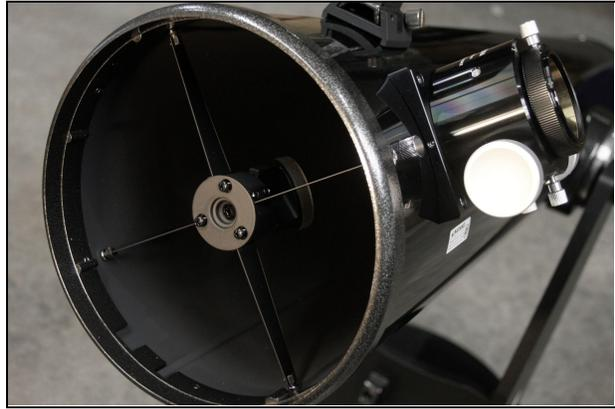
Begin by removing the front cover of the telescope. Then, gather the collimation knobs and screwdriver from the AD Upgrade box. Take notice of the three outer screws on the face of the secondary hub, plus the one central screw. The central screw should never be tightened or loosened unless there is a very good reason to do so.
