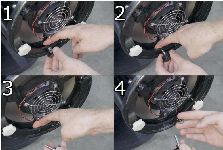
Replace the spring, holding it between two fingers much like what is demonstrated in the last step of the above image, and then insert the knob. Tighten the knob several turns but do not completely tighten it. Repeat the above process for each of the remaining springs. If you have trouble engaging the threads of the knob that you are installing due to the primary mirror cell being too far away, try tightening one of the other black knobs a turn or two – then try again.
