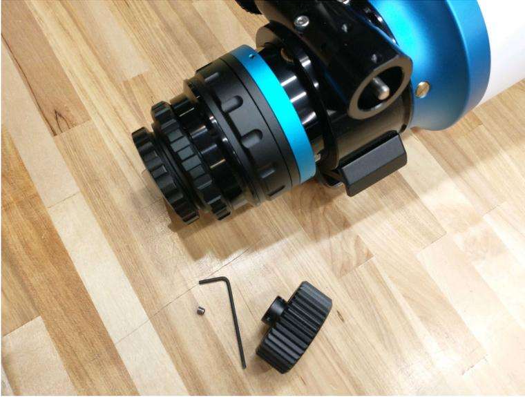
6. Locate and install the 6mm flex coupling that would have been included with the EAF. Install this in place of the coarse focus knob, in the previously mentioned steps in the reverse order.
