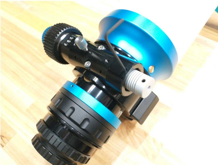
7. Remove the focuser lock knob from the bottom center of the focuser.
