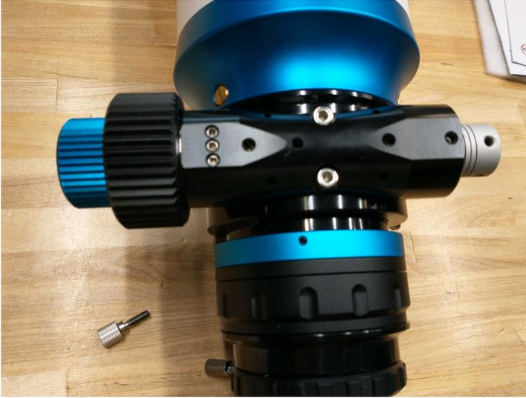
8. Sit the EAF bracket on top of the focuser block where the focus lock knob was installed, with the L bracket facing away from the telescope.
