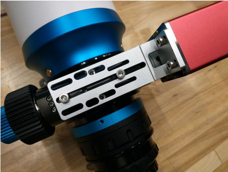
11. Adjust the lay of the bracket and focus motor until it appears to be square and true.
