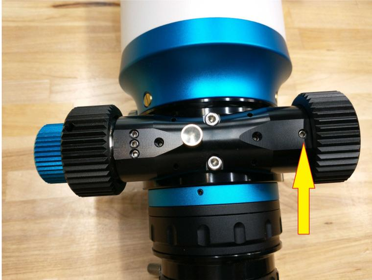
3. Then, rotate the focuser knob until a similar black set screw can be seen through the hole previously occupied by the silver screw. Using the 2mm hex key, loosen but do not remove this screw. If the screw is turned more than necessary it will jam against the focuser housing and prevent the knob from being removed. A single turn counterclockwise is all that is necessary to remove the focus knob.
