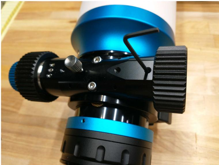
4. Rotate the focuser shaft 90deg from its current location to locate the next 2mm black set screw and loosen this screw, but do not remove it.
