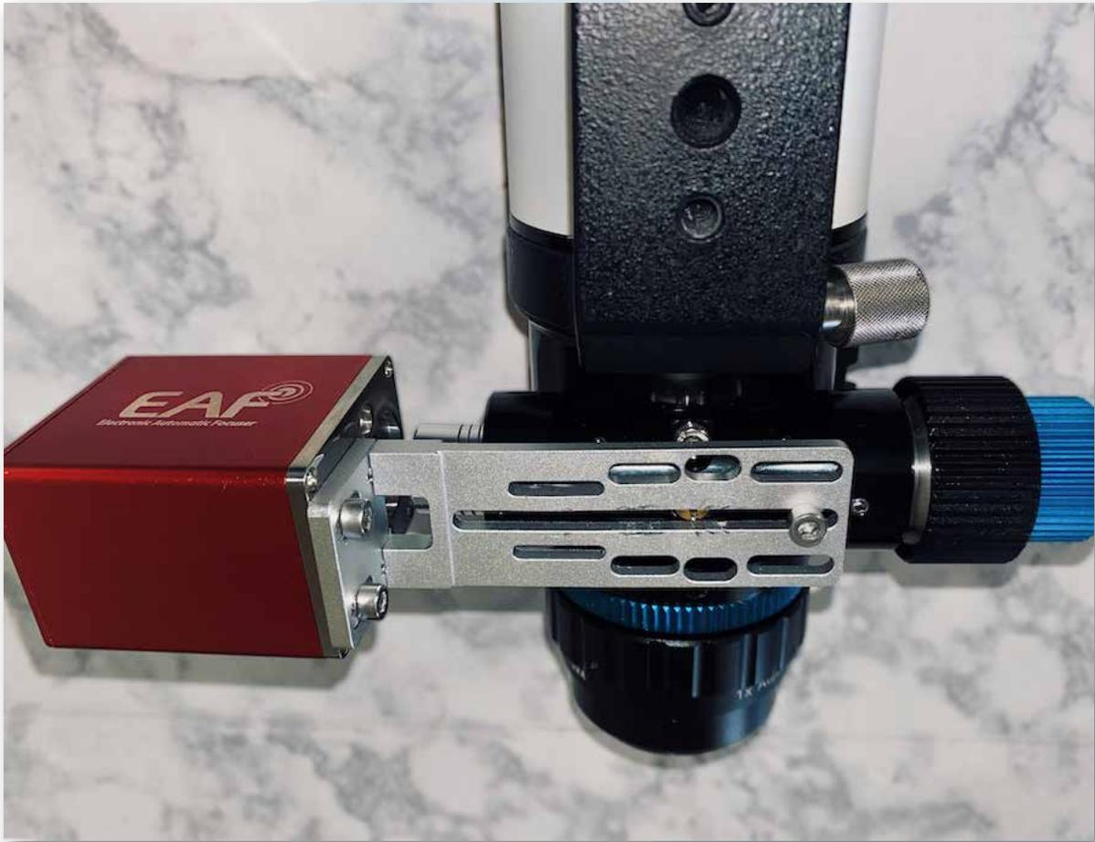
The ZWO EAF is compatible through the coarse adjustment knob.
