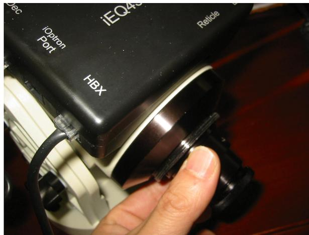
2. Point the Polar Scope to a far distant object. Adjust the Objective Lens by turning the tube to get a clear image. Tune the lock ring to secure it.
