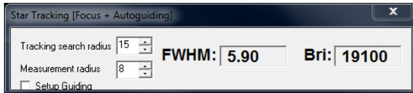
Press the Loop button to begin taking repeated exposures and adjust your telescope's focus until it's at an optimum level both visually and with the maximum and minimum values.
