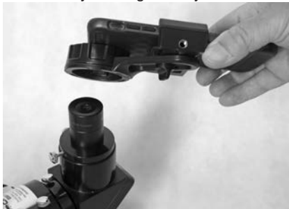
Figure 5. Place the turret over the eyepiece of your instrument (a) and turn the turret's twist-tight housing until it firmly grips the eyepiece (b) .
