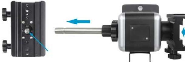
Slide the counterweight (optional) onto the CW shaft **with large opening hole facing inward**. Insert the brass pin into the hole on the CW. Secure the CW by tightening the CW lock knob. (The groove on the CW shaft is designed for secondary dovetail saddle use.)
