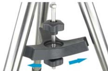
6. **Attach Telescope:** Attach a telescope to dual dovetail saddle. Make sure that the telescope objective end is pointing to the direction as the arrow mark on the dovetail pointed to. The dovetail saddle can be rotated freely when the altitude lock knob is released. Fully tighten the altitude lock knob afterwards.
