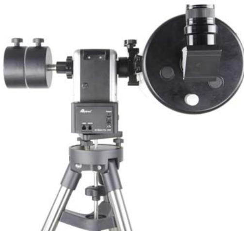
A simple and safe method to estimate the CW and its position is by calculating the torques (*weight times the distance to the center*) of the payload and CW, and making them equal or close.
