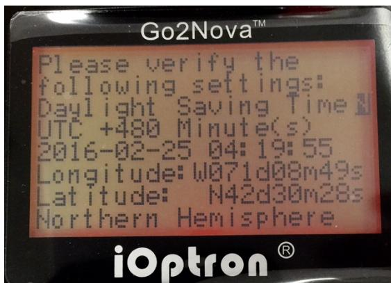
If all the information is correct, you may press **ENTER** to confirm and skip waiting for GPS signal. Or if the mount could not pick up the GPS signal (the mount won't advance to next step to start slewing), you can manually change it by setting Daylight Saving Time (DST) to Y(es) or N(o); adjusting the date and time; inputting your location coordinates; entering the time zone offset to the UTC; for examples:
