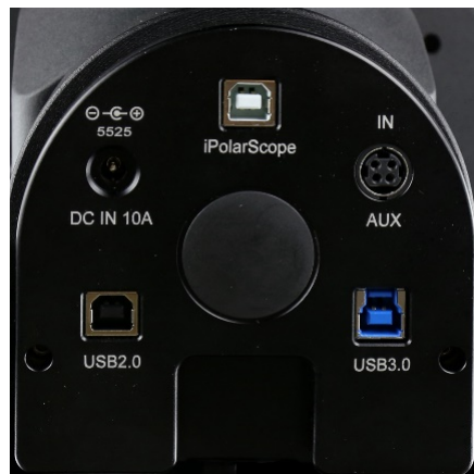
Figure 7. Cable Management System Input Panel
