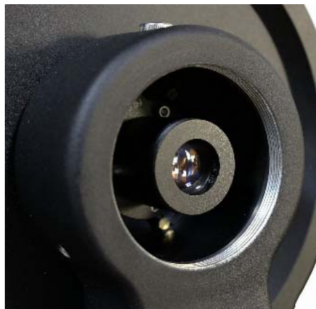
Figure 17. CEM120 with an installed electronic polar scope
