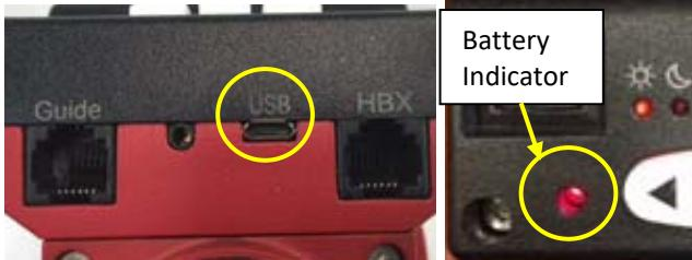
**⚠️** Please don't charge the battery or use USB power when temperature is at or below 0°C (32°F), otherwise the rechargeable battery might be permanently damaged.
