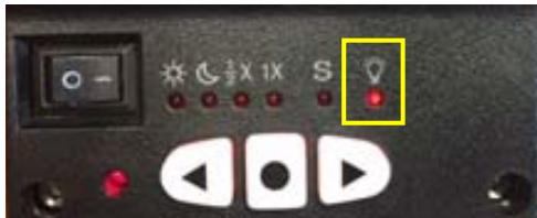
When done light intensity adjustment, double check the LED under letter "S" to make sure the correct hemisphere is selected.
