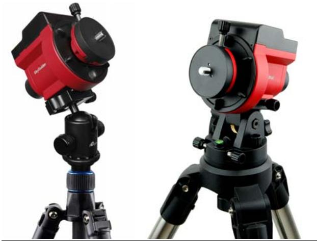
To use the alt-azi base, just simply slide the mount head base into the alt-azi base dovetail saddle. You can slide the mount head in from either direction depending on your latitude position and payload. The latitude adjustment range can be from -40° to 60°. If possible, choose the one with the center of gravity of the system as close to the center of the base as possible.
