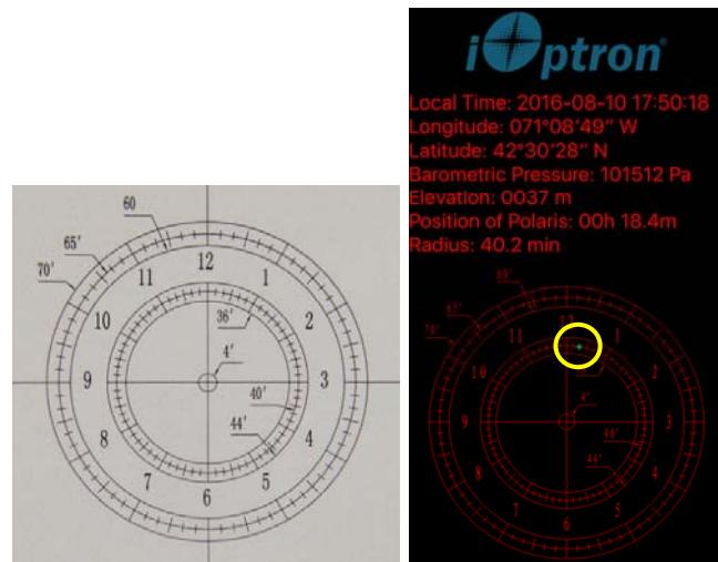
Press the power switch on the mount to turn on the mount. Look through the polar scope eyepiece. If you can not see red polar scope dial or 12 o'clock mark is not on top, release RA Clutch Disk slightly. Rotate the RA axis until you see the red LED illumination and/or adjust the 12 mark to the top. Lock the RA axis again. Adjust the eyepiece to bring the reticle dial in focus.
