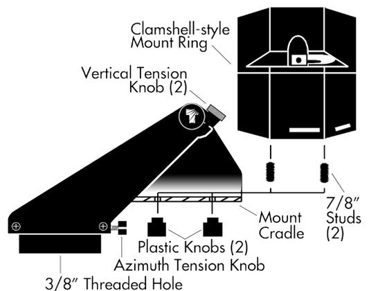
**WARNING:** Rotating the Tele-Pod head while the azimuth tension knob is tightened could cause the azimuth bearing to unscrew and separate.
