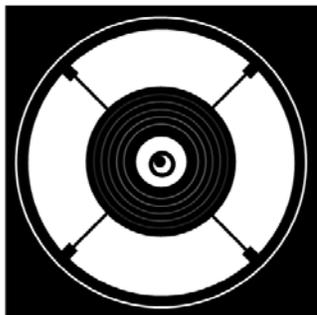
There are three collimation set-screws at the front of the secondary mirror holder. This will adjust the tilt of the secondary, changing the relative position of the secondary center ring when peering through the collimation eyepiece.
