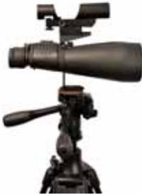
If your binoculars are attached via a photo screw on the front of the middle bridge and an angular or L-adapter on a tripod, attach the SkySurfer III on the adapter ⑥. Run the fastening screw of the tripod adapter through the hole of SkySurfer adapter and screw both on your binoculars. So you can use the SkySurfer also with large binoculars with a small field of view. On binocu-
