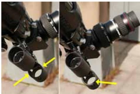
On the right is the sight when the sun is not centered and the shadow only cuts the rear ring (yellow arrow). You may need to re-adjust the viewfinder for solar observation, or mark the intersections of the shadow on the rear section. Please follow the safety instructions of your telescope when you observe the Sun. You can find safe solar filters on <http://astrosolar.com>.
