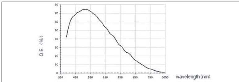
**Figure 10.** 74% High Quantum Efficiency (QE) of the **SAGPRO**.
