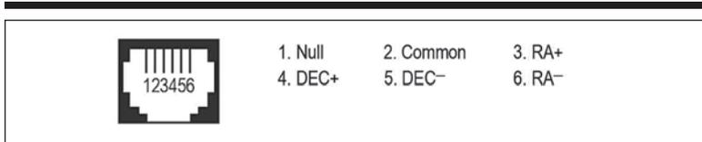
**Figure 9.** Pin out diagram for ST4 Port.
