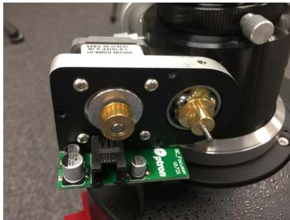
3. Put the eFocuser pulley onto the dual-speed focuser tuning shaft. Tighten the set screw so it is sit on to the flat surface of the coarse tuning shaft.
